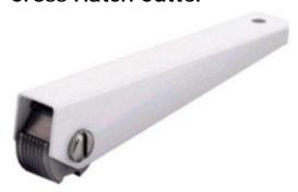
The Cross Hatch Cutter will allow an assessment to be made of the adhesion resistance of coatings to separation from substrates when a right-angled lattice pattern is cut into the coating and penetrates through to the substrate. The coating thickness determines the Cutter size used. The 1mm Cutter is suitable for coatings under 60 microns; the 2mm cutter is suitable for coatings over 60 microns.
