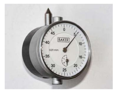
> Crankshaft Gauge measures the Web deflection of a Crankshaft.
