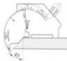
Misalignment in Butt Weld
