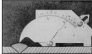
EXCESS WELD METAL
