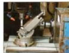
The Angular Machine Vice being used for 45° face milling
