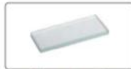
50mm reading scale (check magnification accuracy)
